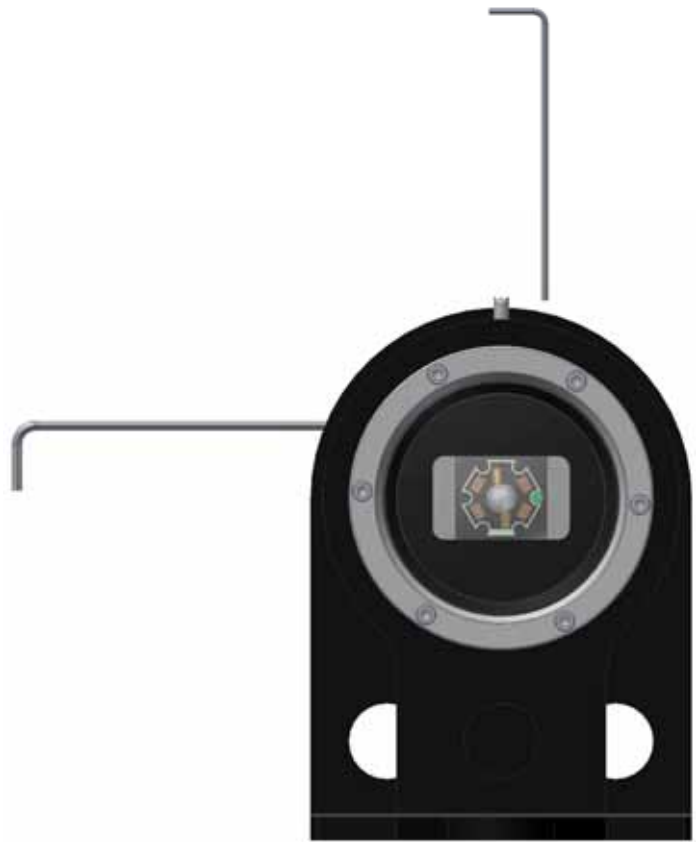
FRONT VIEW FOR APERTURE PLATE ADJUSTMENT
